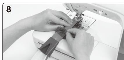
Keep the position of paired units A/B and C/D close to the needle plate and slide along as you sew.
