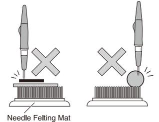
• Do not remove the needle at a different angle from when it was inserted as this may cause the needle to break.
